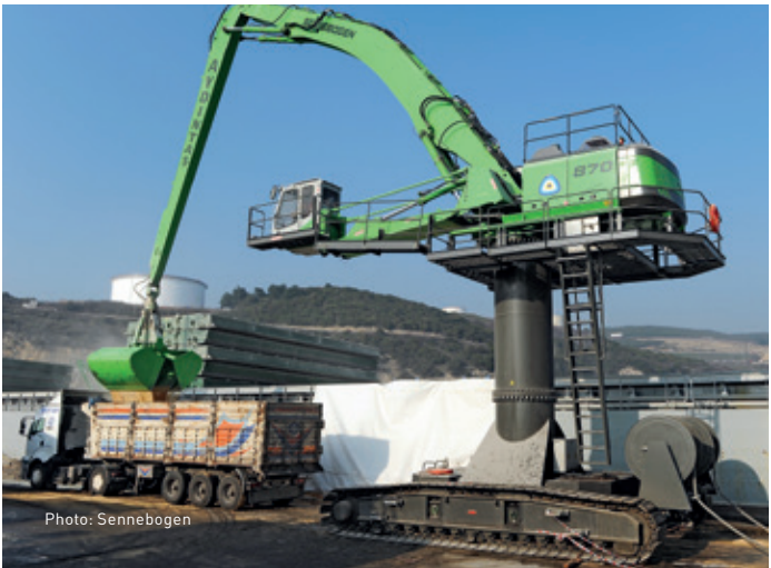
Spiral cable reel mounted on a crawler undercarriage. Suitable for higher travel speed and sufficient installation space upwards. Power transfer from cable reel via slip ring assembly in the centre of the pylon to the motor (M).
